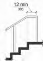
FIGURE 11B-505.10.2 TOP HANDRAIL EXTENSION AT STAIRS
