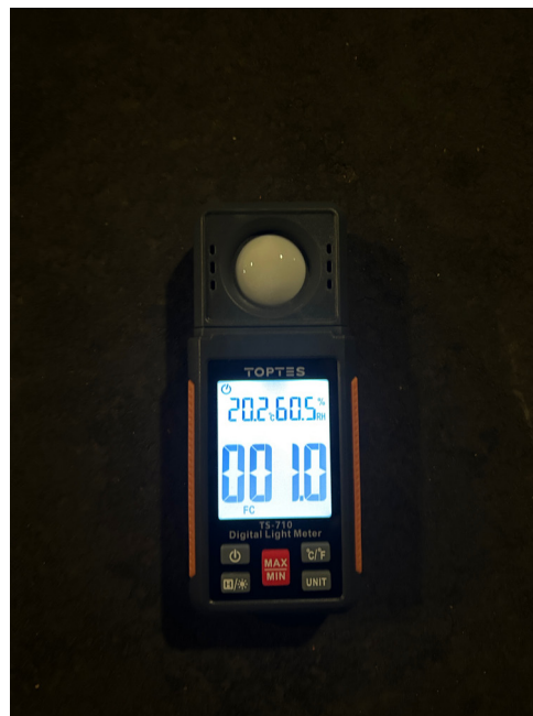
Maravilla retirement community car ports. Meter reading is 1.0 fc at brightest spot.
