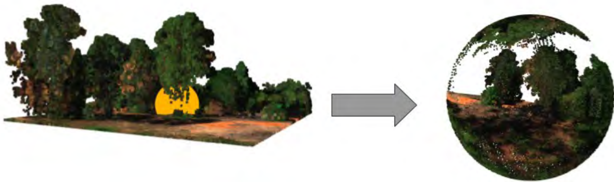
Figure 23: An example of a point cloud projected to a sphere. The yellow sphere located in the center of the unmodified point cloud (left) represents the center of the sphere and the point of view for the simulated photo.
