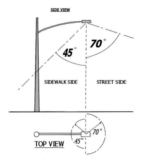
Figure 1 – Tree Trimming for Streetlights
