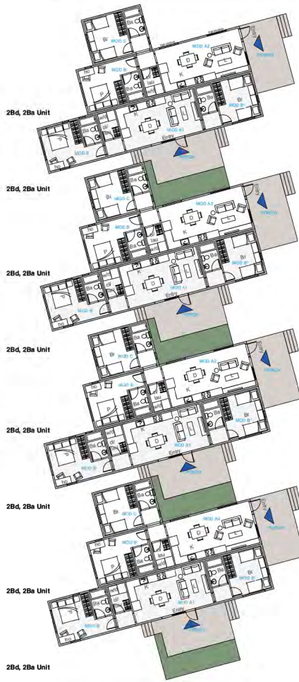
EIGHT UNIT (4 Duplex) CONFIGURATION (8) 2 Bd, 2 Ba Units 8 Total Units, 16 Bedrooms, 16 Bathrooms, 8 Kitchens Staff Housing Proposed Plans (2)
