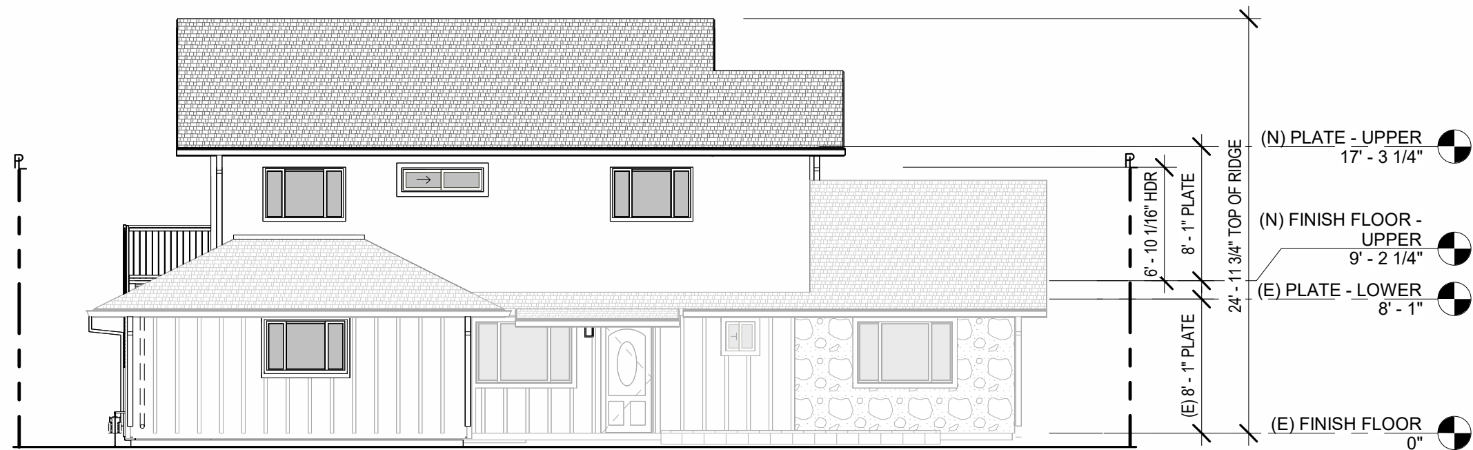
① SCHEMATIC SOUTH ELEVATION - DRB 1/8" = 1'-0"
