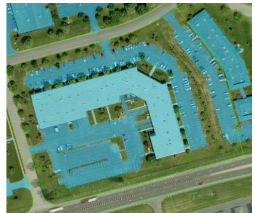
Example of digitized impervious area for a non-single family residential property. Measured impervious area is shown in translucent blue.
