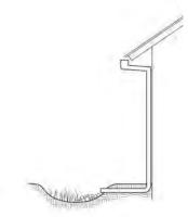
Connecting a roof leader to a vegetated area. The head from the eave height makes it possible to route roof drainage some distance away from the buildina.
