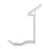
Connecting a roof leader to a vegetated area. The head from the eave height makes it possible to route roof drainage some distance away from the buildina.
