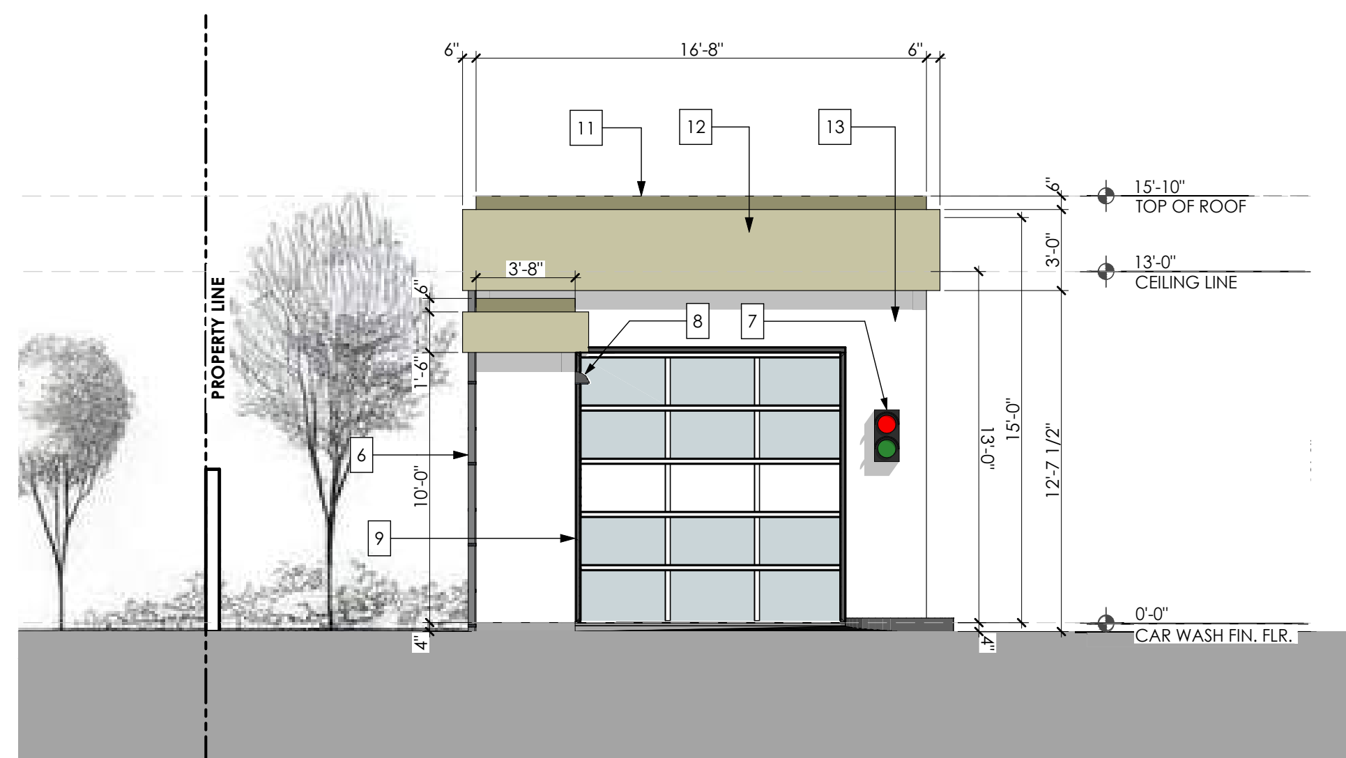
E-03 CARWASH EAST ELEVATION 3/32" = 1'-0"
