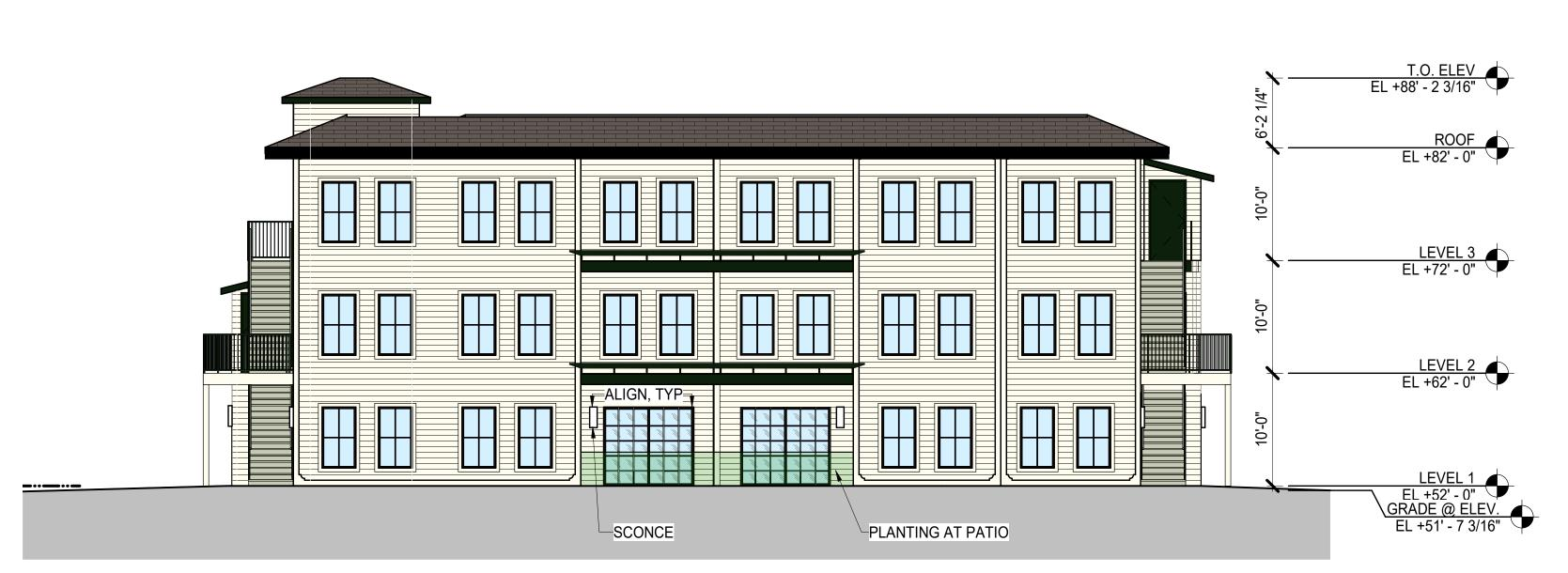
**SOUTH ELEVATION - PROPOSED** SCALE: 1/8" = 1'-0"
