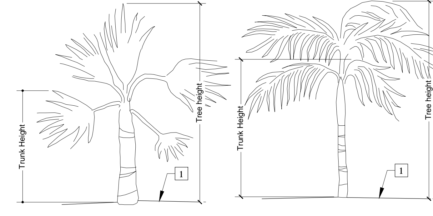
6 TRUNK HEIGHT DEFINITION Not to Scale
