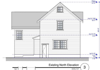
Existing North Elevation 3
