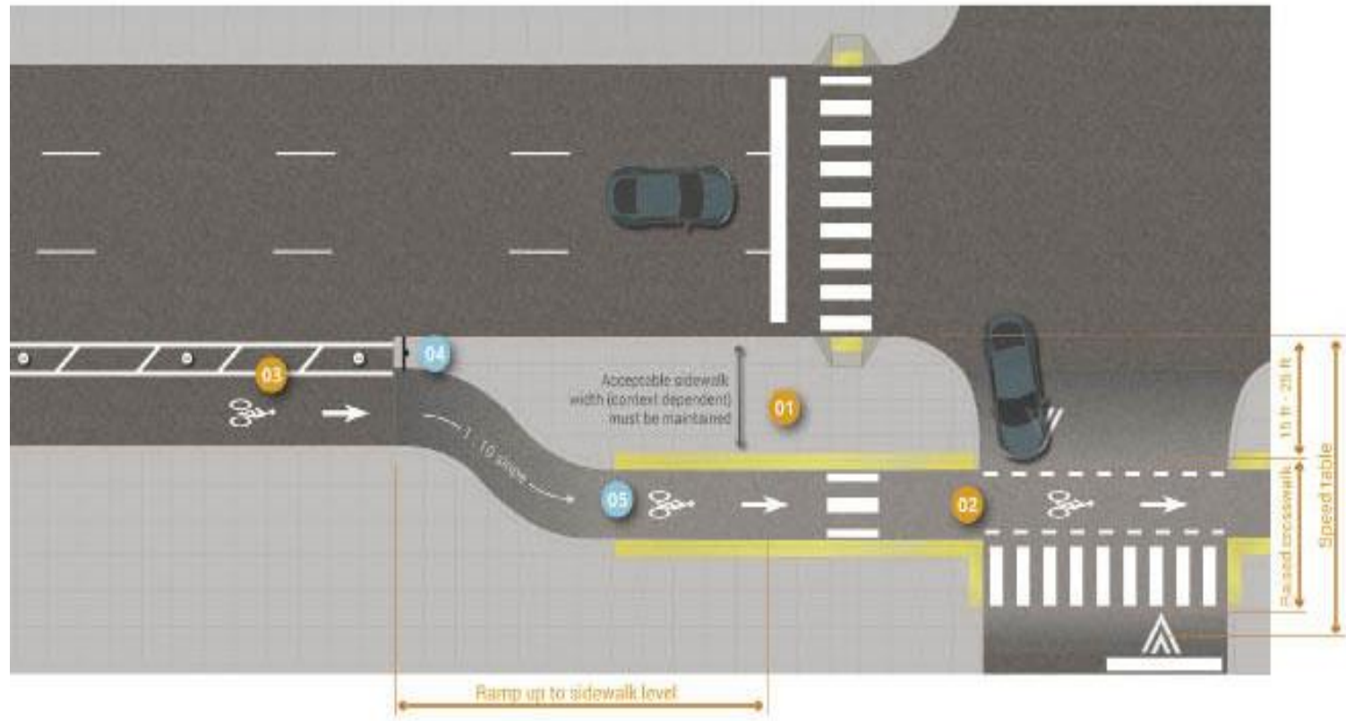
Figure 2 – Typical Bend Out Design with Speed Table (FHWA Separated Bike Lane Planning and Design Guide)
