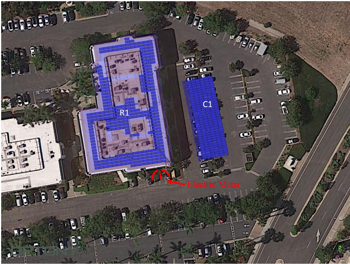
Figure 2: Goleta City Hall Recommended Solar PV Design Layout (Yield = 1,625 kWh/kW)
