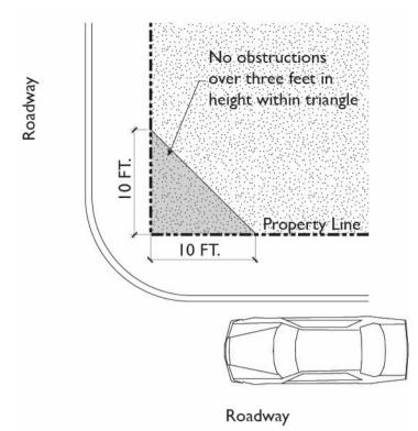
I. Subsection 17.24.210(A)(2) of the Goleta Municipal Code is amended to add "FIGURE 17.24.210(A)(2): CLEARANCE TRIANGLE, DRIVEWAYS" as shown below:
